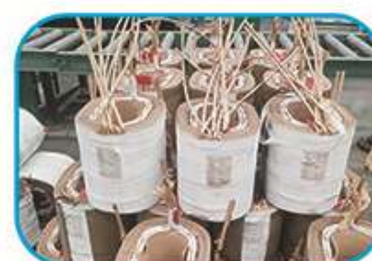
Winding for Oil Transformer
